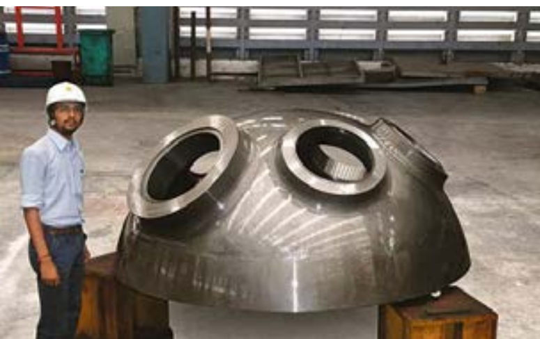
Dished ends forged at L&T's forging facility at Hazira, Gujarat.
