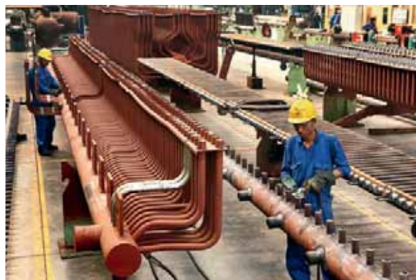
Supercritical boiler manufactured at the state-of-the-art manufacturing facilities in Hazira.
