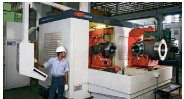
Five-axis machining centres ensure dimensional accuracy and consistency
