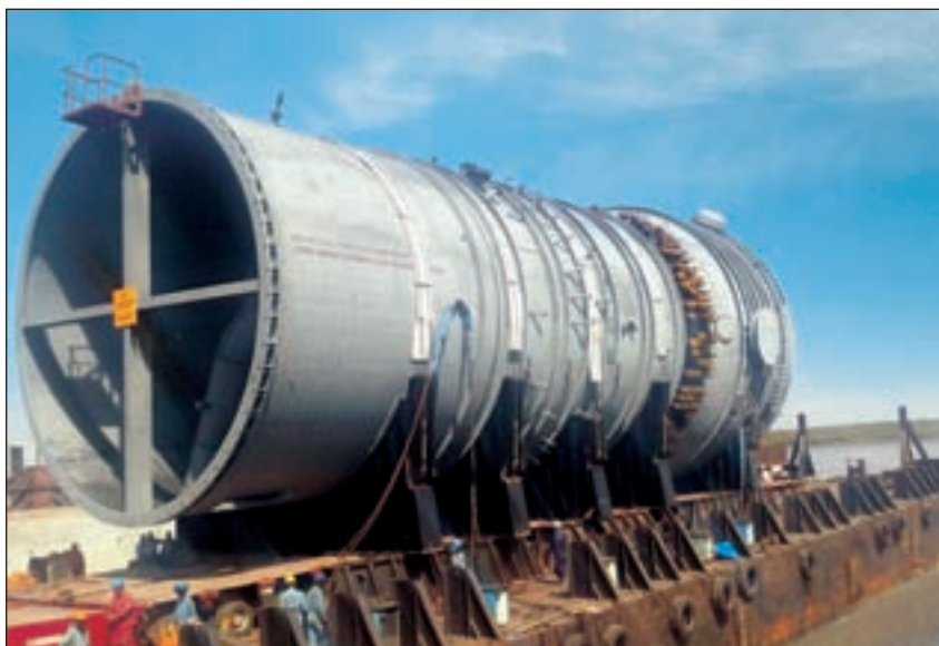
Acrylonitrile reactor – one of the world's largest – for a petrochemical plant in Thailand.
