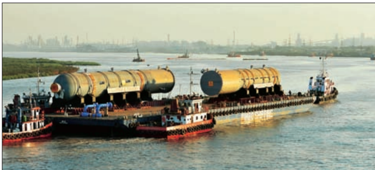
'Clean Fuel' reactors being despatched from L&T's Hazira Works for Kuwait National Petrochemical Corporation.
