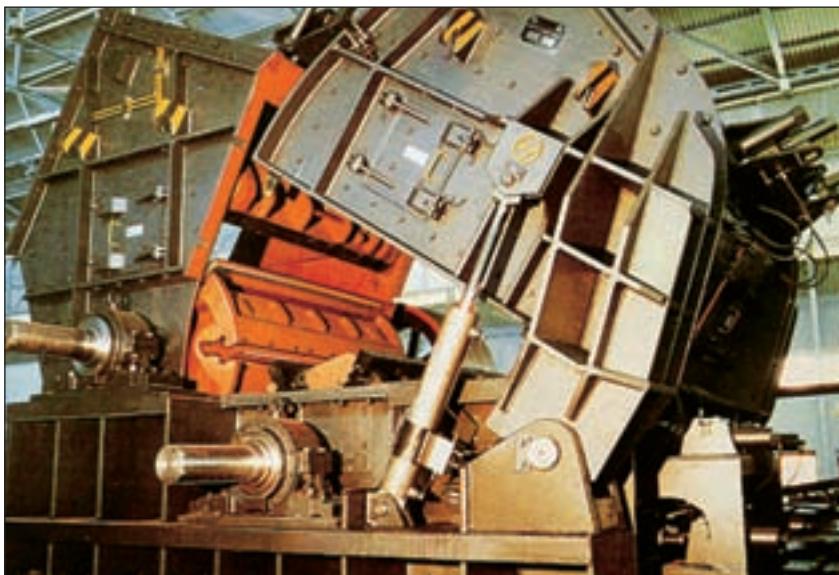
Limestone crusher manufactured at L&T's Kansbahal Works, Odisha
