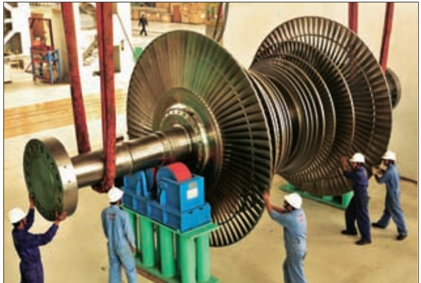
Supercritical turbine under assembly at L&T's Hazira campus.
