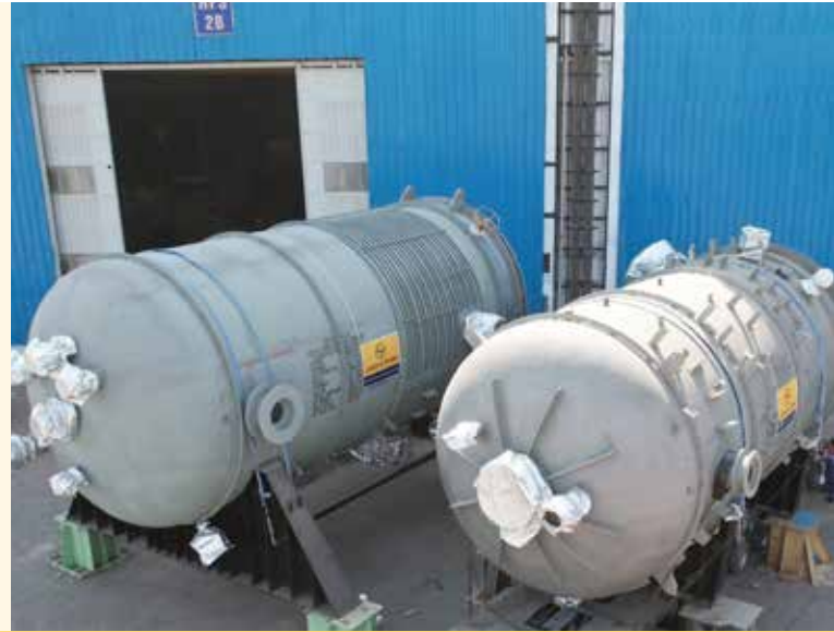
TA Crystallizer and PTA Crystallizer for Mega PX-PTA project at IOCL Paradip Refinery, Odisha
