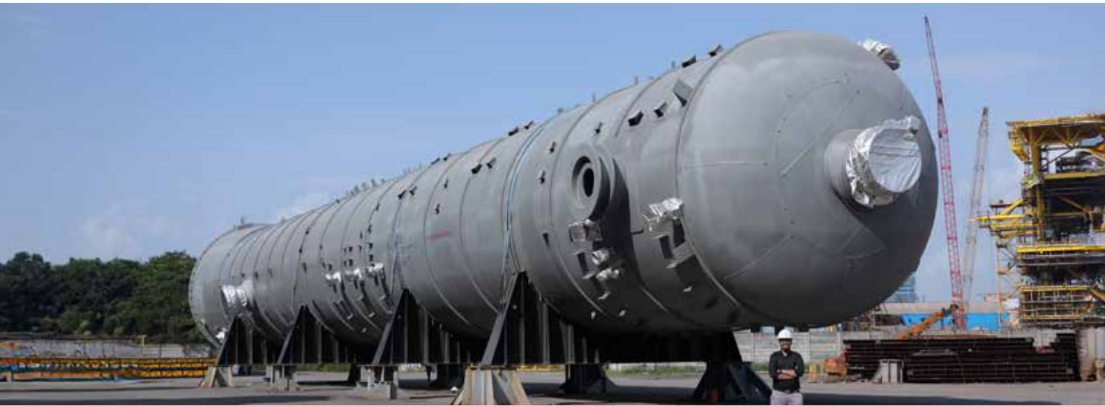
HDS Reactor for IOCL Panipat DHDT project, Haryana
