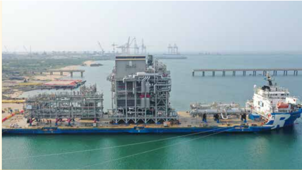
Modularised Reformer for a Blue Hydrogen project in Rotterdam, Netherlands
